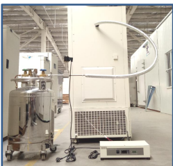
LN 2 /CO 2 backup system
